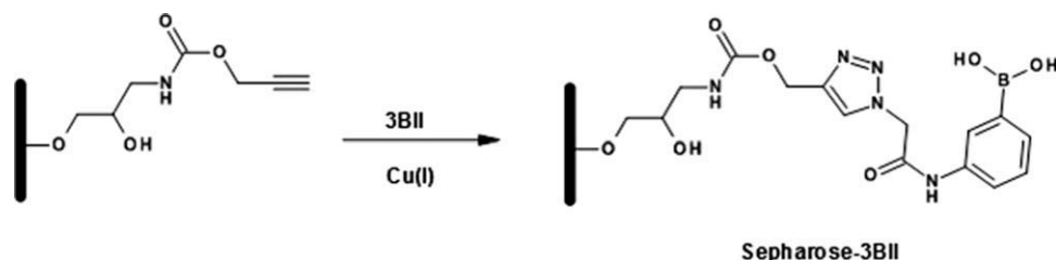
Figure 9. Immobilization of 3BII using CuAAC.
